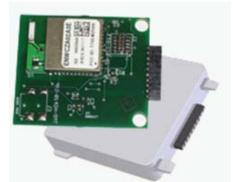
The user-replaceable U-SNAP module shown here measures only 1.5 inches (3.8 cm) square. The plastic enclosure protects the circuitry while providing convenient access from the exterior of the device. A HAN Device Portal designed to use plug-in U-SNAP modules offers the consumer greater flexibility while offering the utility a future-proof approach to the HAN.
